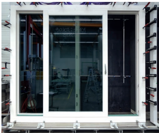
The vinSlide sliding system was tested in the International Technology Centre ITC in Leinfelden-Echterdingen.
